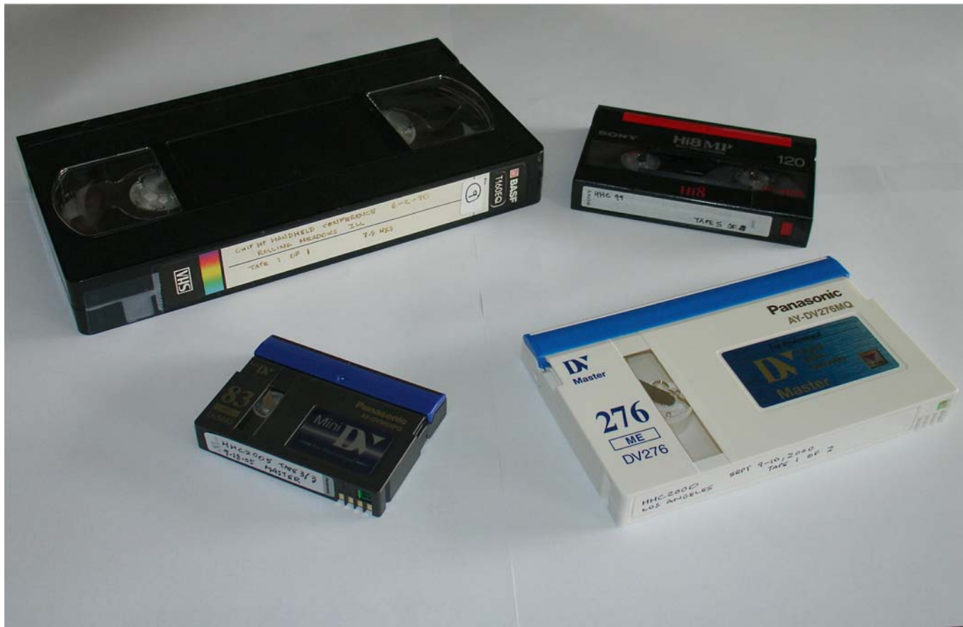
Figure 1. Varying analog and digital tape formats. Clockwise from top left: VHS (analog), Hi8 (analog), full-sized DV (digital) and miniDV (digital).
