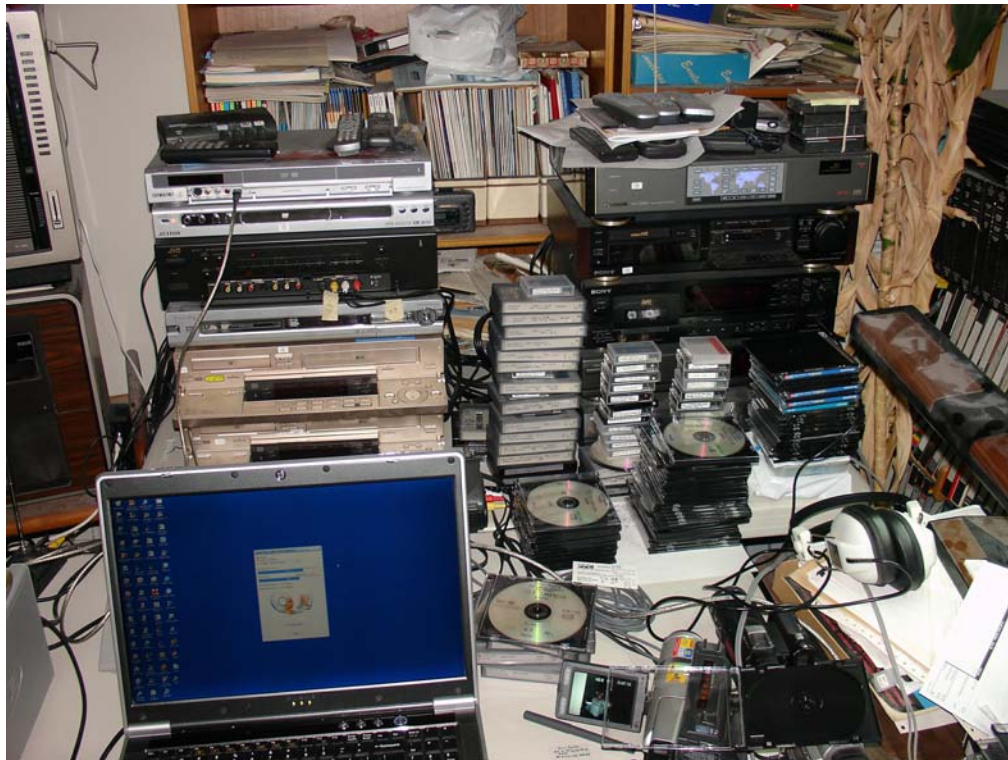
Figure 2. The tape editing, DVD recording and copying equipment. Camcorders are used as playback decks in order to convert the analog tapes to large-format DV tapes.
