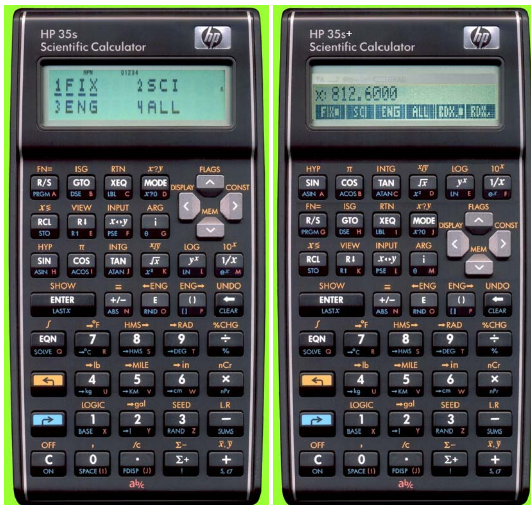
Figure 2. HP35s and a fictitious “35s+” with the third row of keys moved up to row one so as to enable an HP42S-like LCD and soft-key menus. This would be my “fantasy” 35s.
