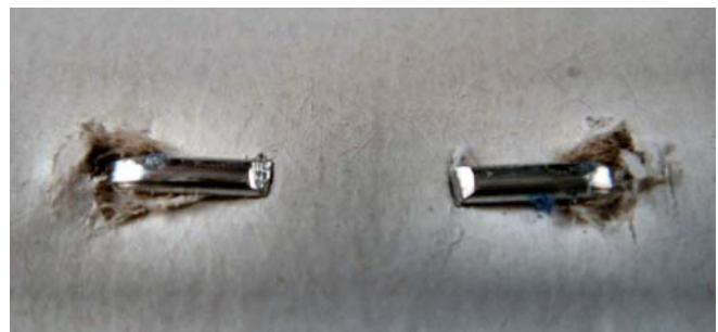
Fig. 9 - Staples of figure 8 flattened. Note that the chipboard fibers have been torn from the force of flattening the staple.
